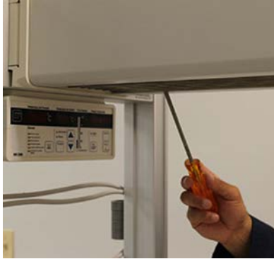
Figure 8: Engaging the Back Reflector Screw
