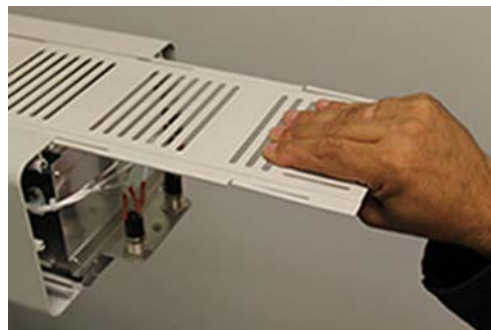
Figure 3: Removing the Ventilation Plate
