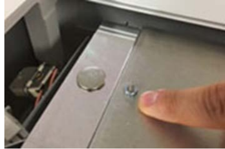
Figure 5: Locating the Back Reflector Screw Nut
