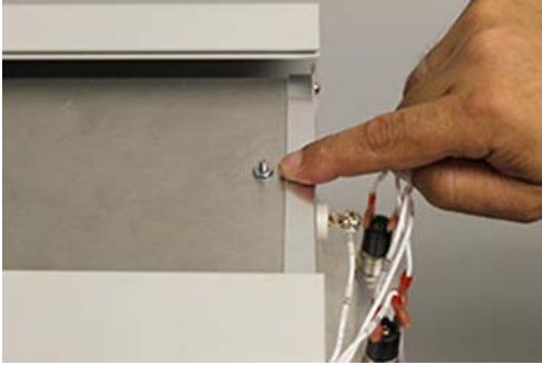
Figure 4: Locating the Front Reflector Screw Nut
